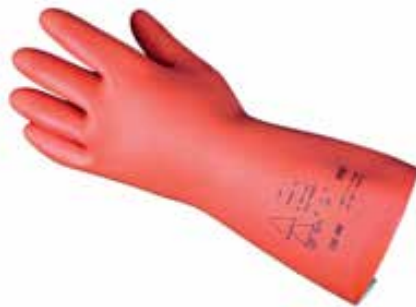
Arc rated insulating gloves, Class 0, ATPV 21.6 or 55 cal/cm 2 CE 0333, EN 60903
