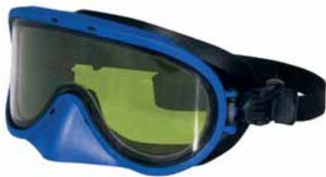
Arc goggles ATPV 12 or 38 cal/cm 2 NFPA 70E-2004, ANSI Z87.1
